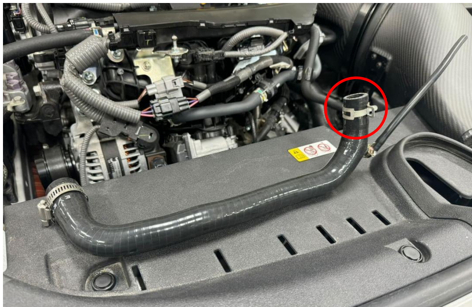
47. Swap over the spring clamp from OEM hose to Eventuri hose at valve cover side.
