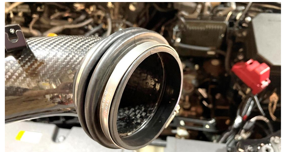
16. Push the hose all the way up to the last visible internal rib of the hose. It should look smooth on the inside like this. Tighten the hose clamp around the tube.
