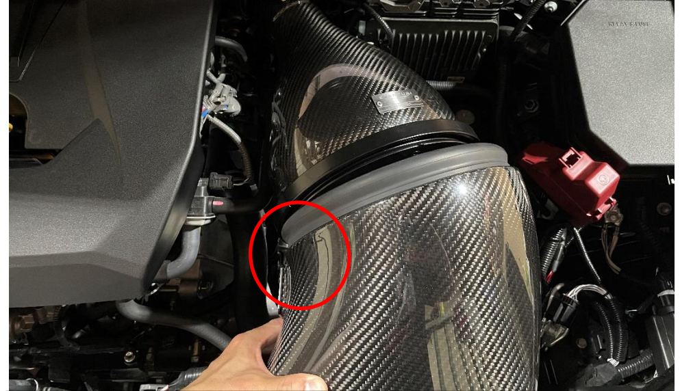
30. Lower the duct into place. The brackets will locate onto the brace shown in the previous step.
