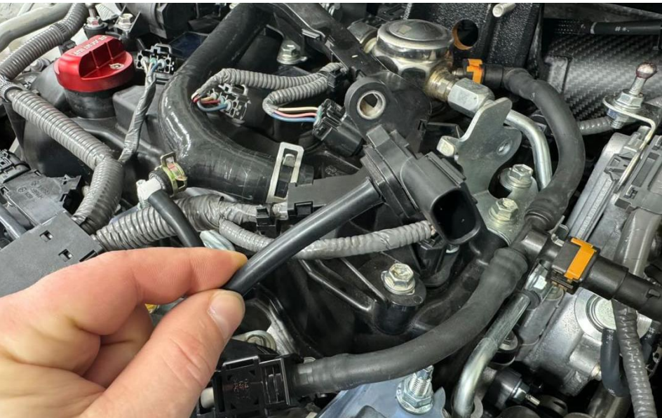
51. Connect the new vacuum line from the Eventuri hose to the crankcase pressure sensor.
