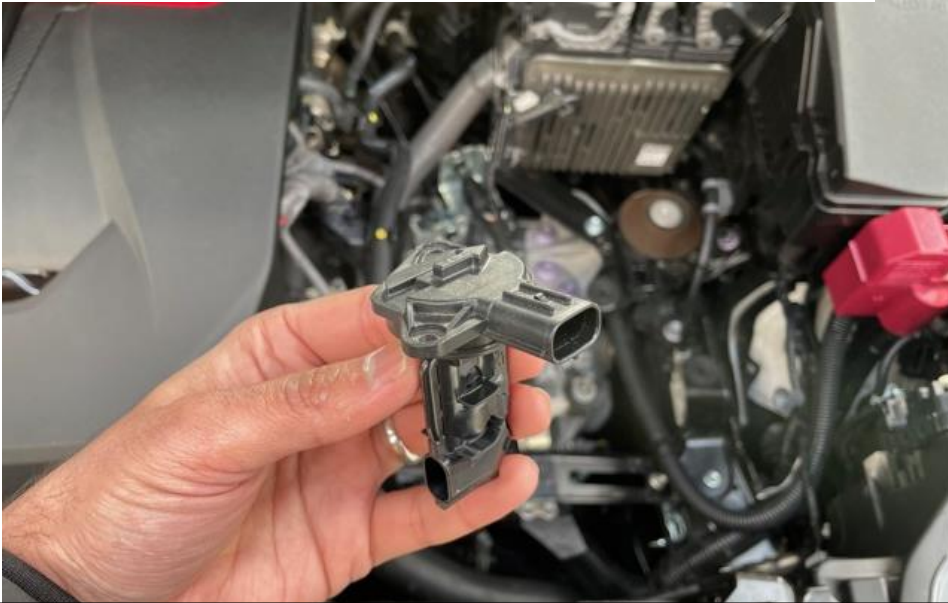
13. Remove the MAF Sensor from the airbox. We will NOT be using the stock MAF screws.
