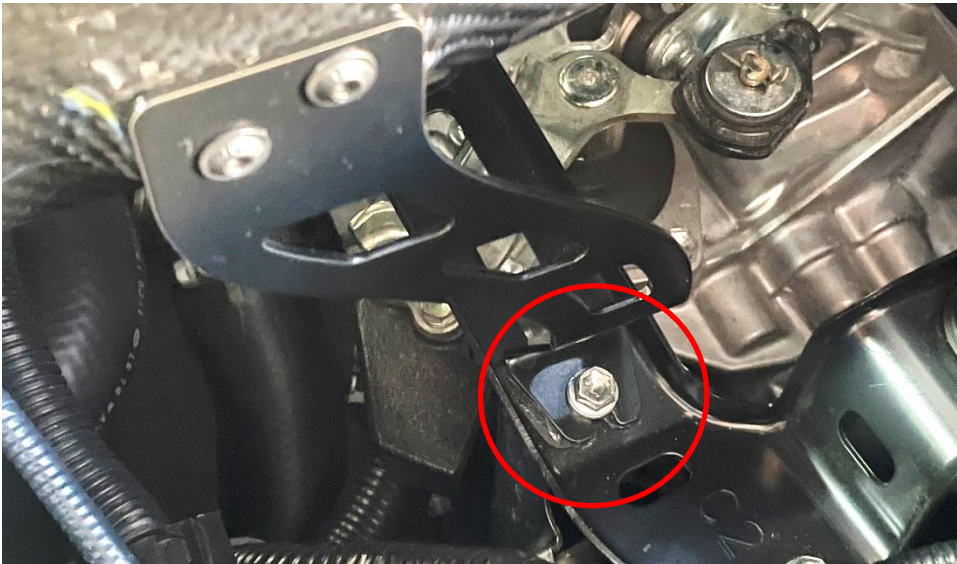
31. Locate the right side bracket onto the brace and secure with the bolt removed in step 25.
