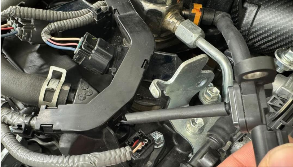
41. Remove the vacuum line from the base of the sensor and also from the valve cover.
