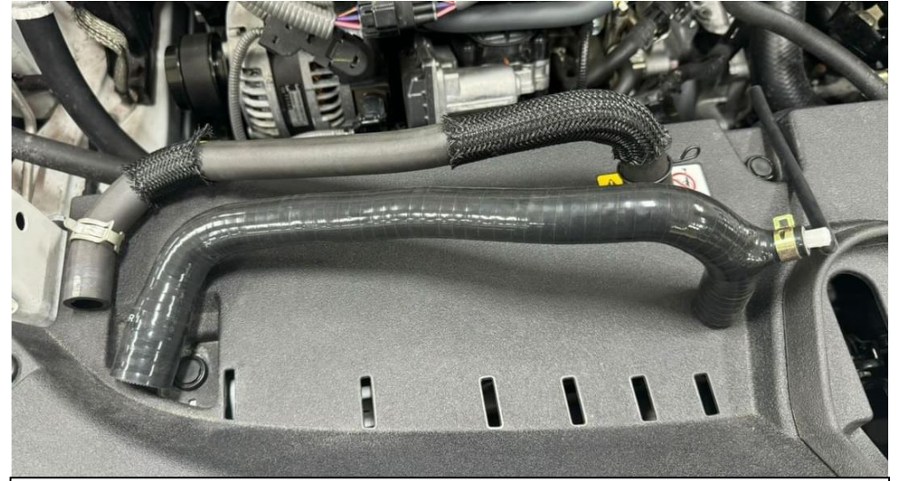
46. Comparison of the OEM and Eventuri hoses.
