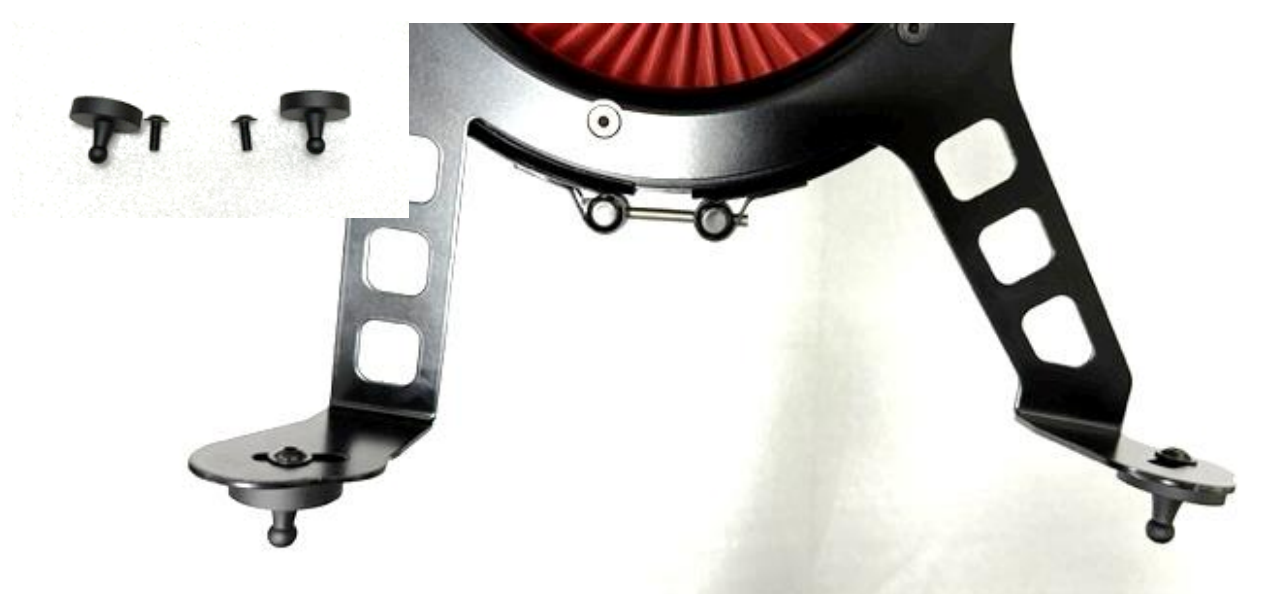
20. Assemble the 2 mounts to the base of the housing bracket using the supplied M5x12 screws and washers. Leave the mounts slightly loose to allow adjustment later.
