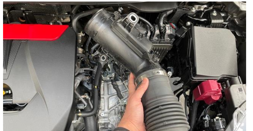
12. Remove the tube from the engine bay.
