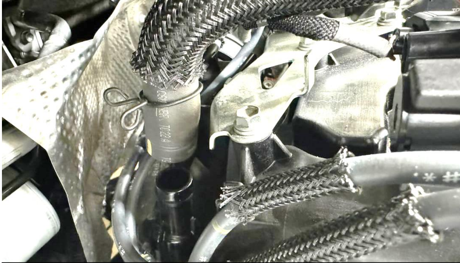
45. Remove the hose at the rear connection to the intake tube. The OEM hose can now be completely removed.
