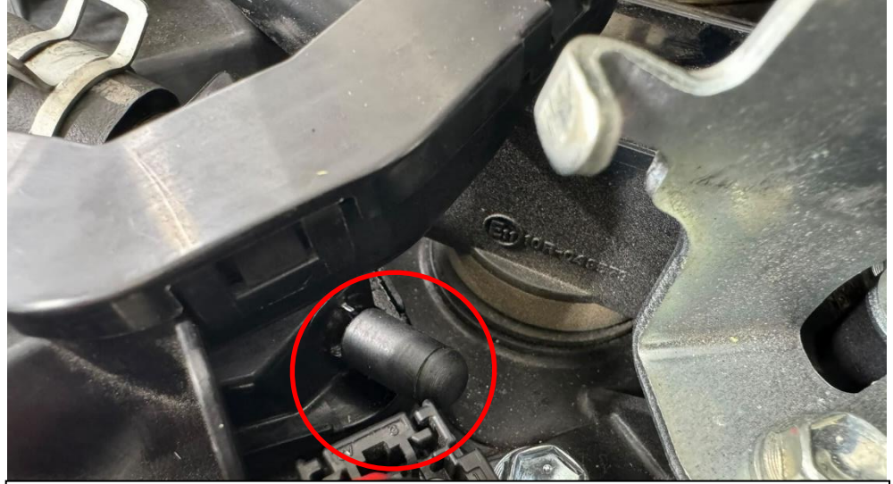
42. Blank off the vac line outlet on the crank case with the supplied cap.
