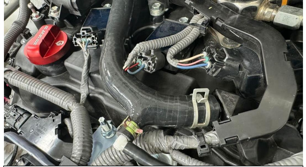
50. Connect the Eventuri hose to the valve cover. Secure with the spring clamp.
