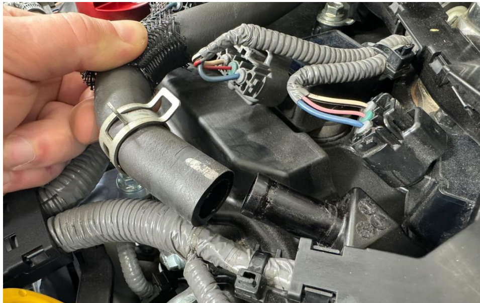
43. Disconnect OEM hose from the valve cover.
